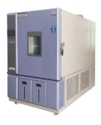
The programmable constant temperature and humidity test chamber is a versatile, essential device. It precisely simulates high/low temperature and alternating humid environments products, materials, and packaging may face during transportation, storage, and use. By exposing them to these conditions, it effectively assesses their resistance to heat, cold, and humid heat, helping manufacturers and researchers spot weaknesses.
